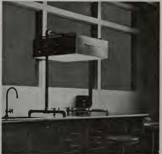
FIGURE 4. Macbeth daylight unit mounted to give even illumination over a large area.
